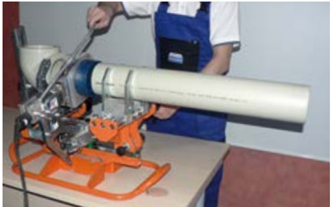
fixing and aligning components in jig, then heating-up
